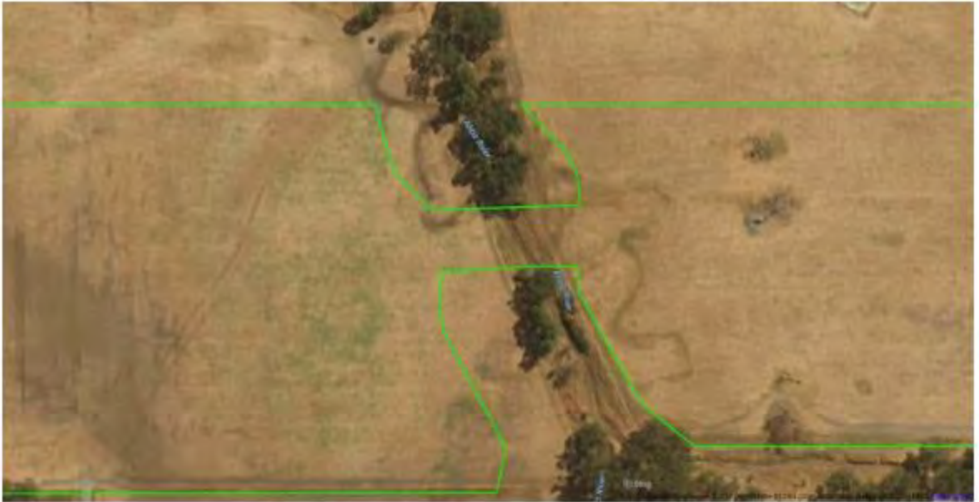
Figure 2: Yalyalup Road access showing reduced width of road at point of Abba River Crossing bridge site to avoid impact on Native Vegetation.
